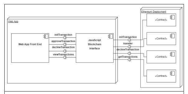
*Figure 3:* A macro-component diagram of how our web application interacts with the smart contracts in our blockchain
