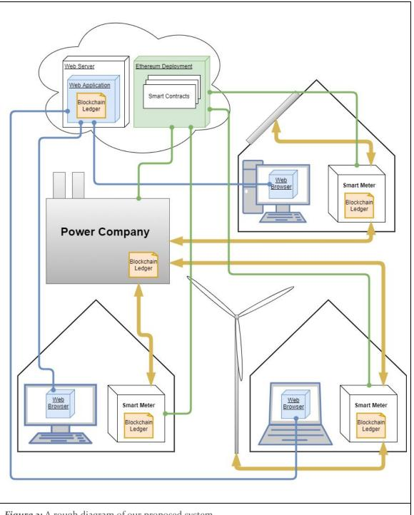
Figure 2: A rough diagram of our proposed system
